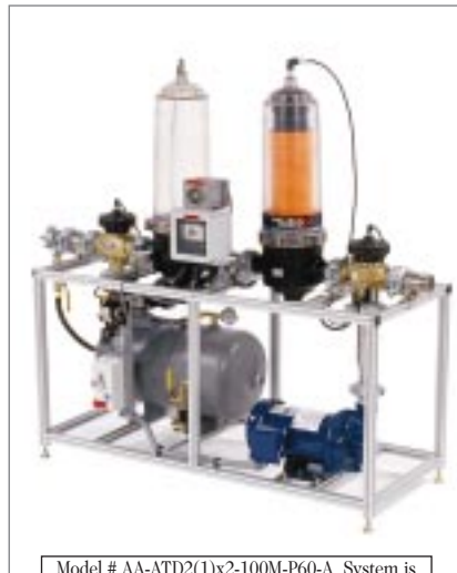
Model # AA-ATD2(1)x2-100M-P60-A. System is rated @ 70 GPM max. System backwashes with filtered water from second filter pod (reservoir).
